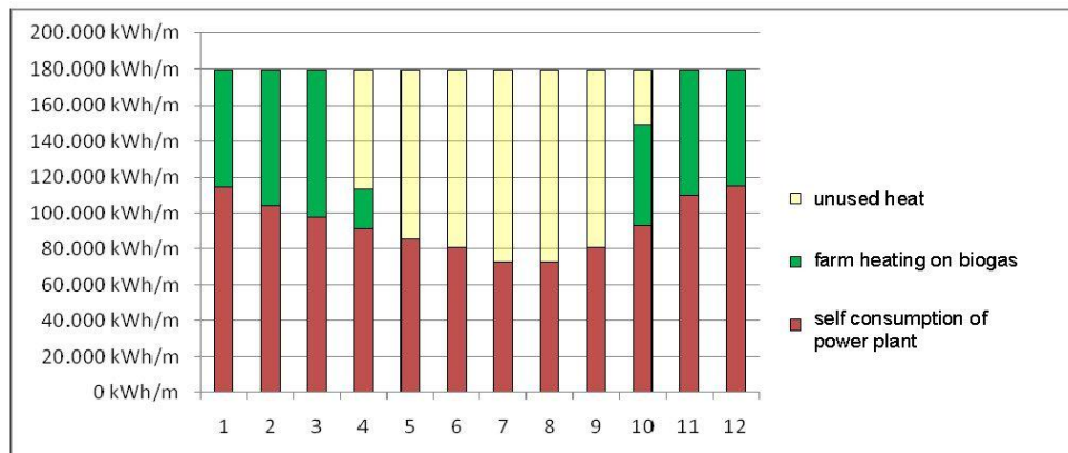
Figure 1. The balance of thermal energy produced in the biogas power plant Vizelj, Serbia
